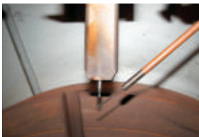
Figure 5. A narrow gap torch with hot wire tube showing the wire angle and position relative to the tungsten.
